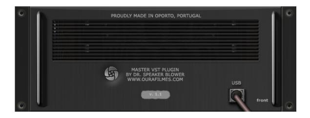
This effect is basically a remix of technologies from 5 processors into 1 plugin: Stereo to Mono (mono), OuraGain (phase reverse), Central Station (m/s), Speaker Blower (limiter) and BassDrive (auto-gain feature). The pan stage is exclusive and is brand new (this is 0dB Center, OuraGain pan is -3dB Center).
