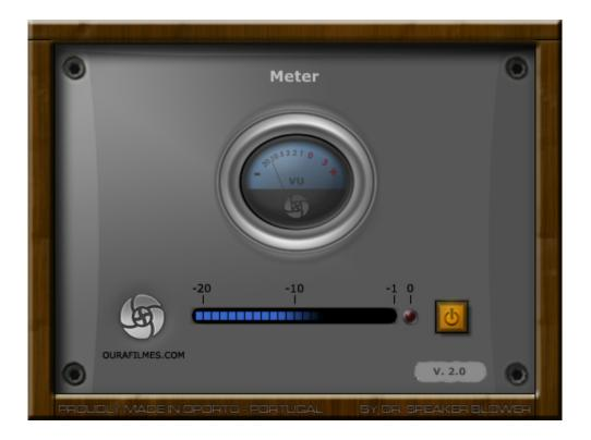
Depending of the situation (or track), use the mono or the stereo components of this vst plugin to analyse and meter the sound level. With RMS, Peak and M/S (and even including a peak limiter spider-eye meter) this is a very complete metering plugin.
