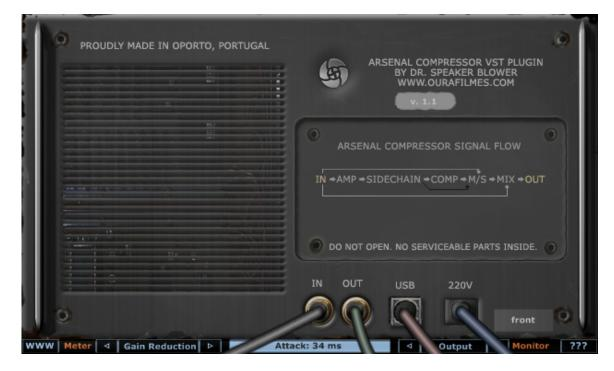
Use this vst effect to process any sound that needs dynamic processing. Use the sidechain feature to process only certain frequencies, leaving the other frequencies unprocessed. And last but not least, with the M/S feature, you can process dynamically only the Mid, the Sides or even achieve parallel compression (50/50) on sides and/or center! This is another future vst classic!
