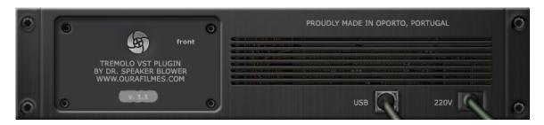
This is a tremolo processor based on a stereo sine wave LFO. With its phase knob, you can control the amount of difference between the left and right LFO start. This allows you to have it from left to right or have both sides in sync. If you turn phase value to 0, the LFOs phase will reset and they start in sync. The filters allow you to only process the sound you plan if you do not want to process all the hearing range.
